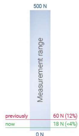
Fig. 1: Effect of full scale value-related errors for measurements in the lower measuring range
