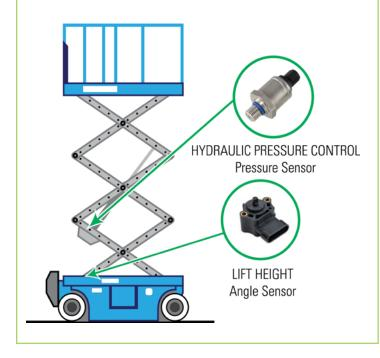
without a good ground connection. In each of these examples, there is an increased risk of electromagnetic emissions that could interfere with the sensor's signal. In such scenarios, specifying sensors that have rigorous EMC standards including Enhanced Radiated Immunity (EMI) ratings of at least 150V+/m and enhanced Electrostatic Discharge (ESD) ratings of ±8kV contact or ±15kV air will help to ensure adequate protection.
