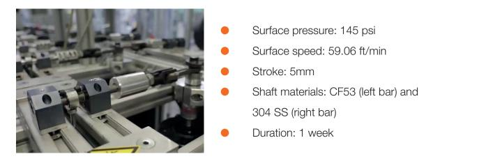
The injection-molded and 3D-printed iglide<sup>®</sup> J260 plain bearings were tested with the same load and surface speeds. Results show that both bearings have similar wear rates, regardless of manufacturing method. The test also shows that our material's coefficient of friction and wear rates are much lower than standard ABS materials.
