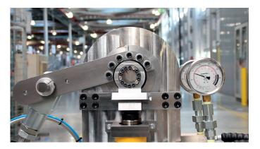
We compared the wear rates of plain bearings made from different iglide<sup>®</sup> materials and manufacturing methods during our pivoting heavy load test. The first was an SLS-printed iglide<sup>®</sup> I3 bearing; the second was a FDM-printed iglide<sup>®</sup> I180 bearing; the third was an injection-molded
