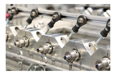
During our pivoting test, we compared the wear resistance of a SLS-printed PA12 plain bearing, a SLS-printed PA12-GF plain bearing, a SLS-printed iglide<sup>®</sup> I3 plain bearing and an injection-molded iglide<sup>®</sup> L280 plain bearing. The test parameters were as follows:
