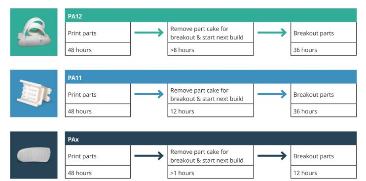
The low printing temperature of DuraForm PAx also enables higher throughput, and its designation as a clean running material reduces operator maintenance, which creates a newfound productivity advantage.
