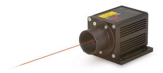
optoNCDT ILR2250 laser distance sensors use the phase comparison method and detect measuring objects at distances of 0.05 m to 150 m with maximum signal stability.
