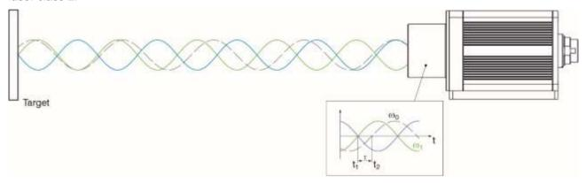
The measuring principle is based on the phase comparison measurement. The sensor emits high-frequency, modulated laser light. The light returned to the sensor is phase-shifted due to the reflection from the measuring target and is compared to the reference signal.
