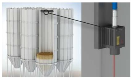
optoNCDT ILR2250 sensors are used for filling level measurements in silos. The laser distance sensors detect the distance to the bulk material or granulate.
