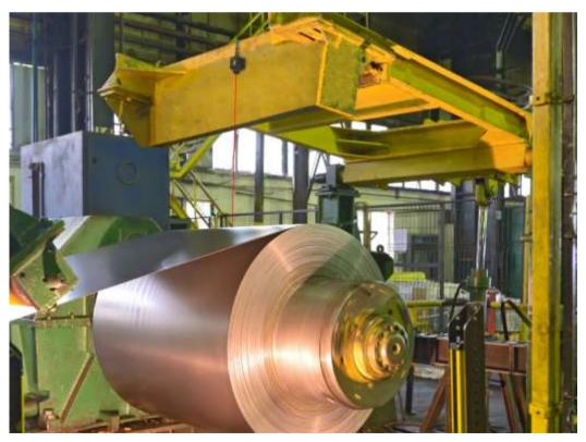
Continuous detection of the coil diameter is necessary in order to monitor the uncoiling process precisely and to determine the changeover time of the coil at an early stage.
