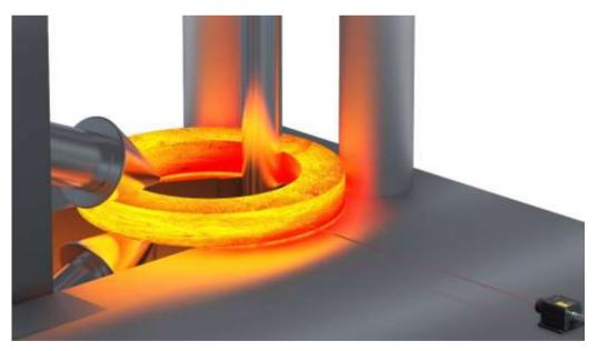
optoNCDT ILR2250-100 laser distance sensors are used for measurements on seamless rolled rings. They operate on the phase comparison method, which provides reliable results even on red-hot glowing measuring objects.
