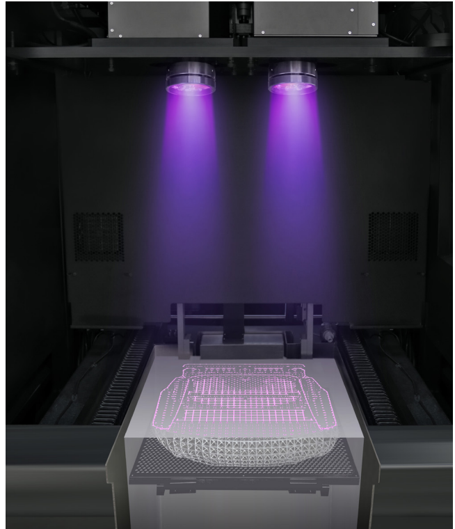
— This is the inside of an Xtreme 8K 3D printing FreeFoam™, a revolutionary expandable 3D printing resin designed for volume production of foam parts. It's part of the DuraChain family of photopolymers printable exclusively on the ETEC Xtreme 8K top-down DLP printer.
