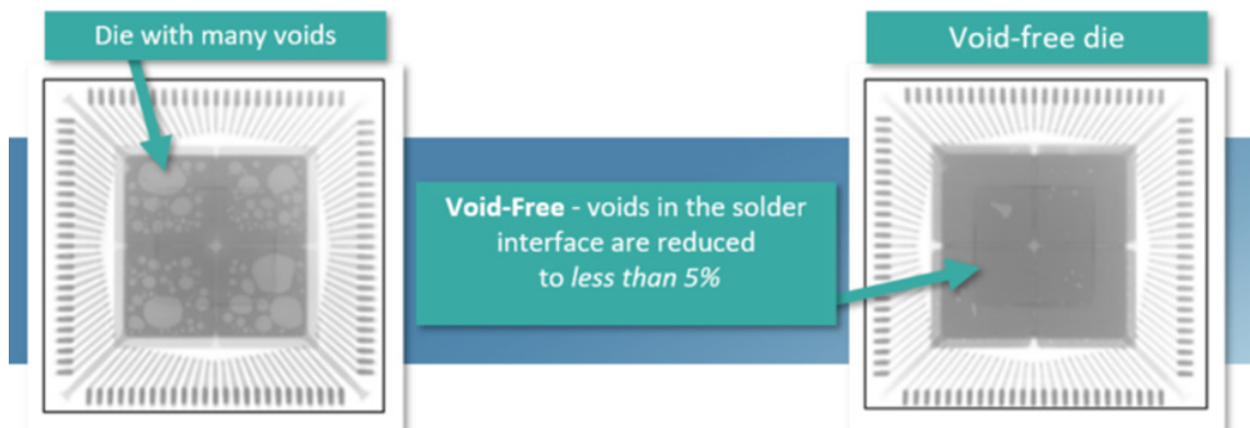
Figure 1: Example of a die with many voids and one with less than 5%, or void-free.
