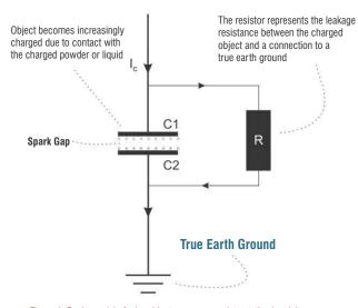
Figure 1: Basic model of why objects can accumulate static electricity.
