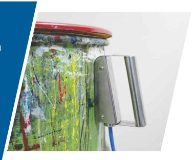
The Tungsten Carbide teeth and torsion spring combination ensure our clamps bite through connection inhibitors like paint, rust, product deposits and ensure a low resistance connection to the metallic object that needs to be grounded.
