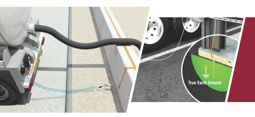
The installation of a truck mounted grounding system requires an experienced EX/HAZLOC electrician who will be able to complete a satisfactory installation that complies with EX/HAZLOC approval requirements and code.
