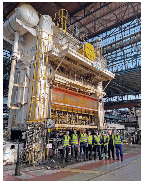
The 4,000-mt press at Maxion Wheels, Czech Republic. [Schuler photo]
