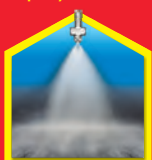
Narrow Angle Flat Fan Spray Pattern
