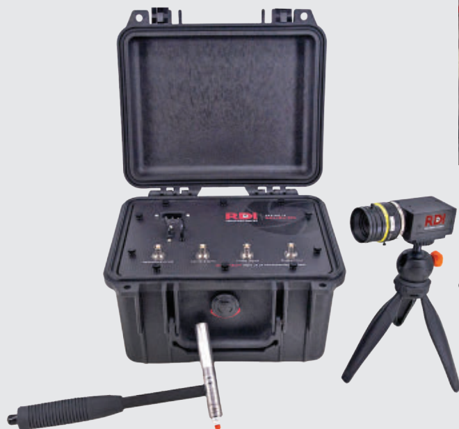
RDI's Modal Amplified system. RDI Technologies
