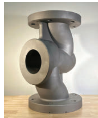
Bechtel Plant Machinery is developing operations to produce additive manufactured components for U.S. Navy nuclear-powered submarine programs. [Business Wire photo]
