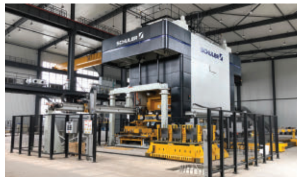
The first Schuler Farina scotch-yoke press has been operating at Strojmetal in Bruntál since 2022. [Schuler photo]
