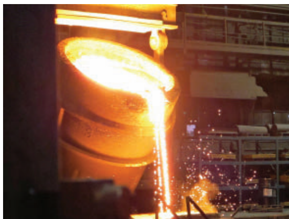
Vacuum processing is critical to producing specialty steel ingots for forging by helping to ensure that the steel solidifies properly, without alloy segregation that would undermine the mechanical reliability of forgings. [ABB photo]
