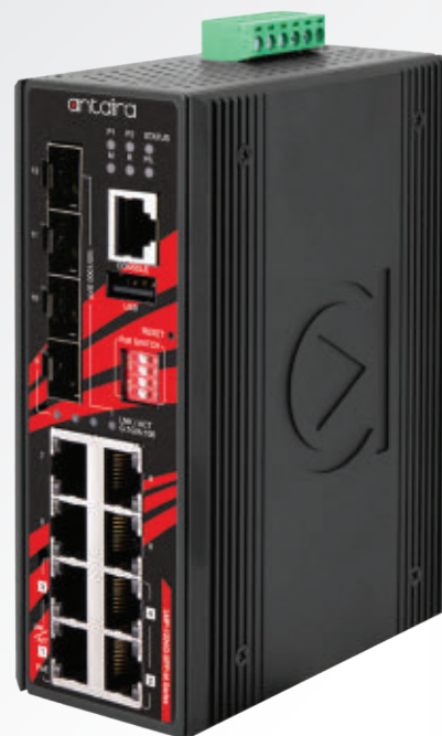
The Antaira LMP-1204G-SFP-bt-24 is a 12-port industrial Gigabit PoE++ managed Ethernet switch embedded with four Ethernet ports that support IEEE 802.3bt for a maximum of 90 W/port, four 10/100/1000Tx Ethernet ports with IEEE 802.3af/at support for a maximum of 30 W/Port, and four SFP slots for fiber connection. © Antaira Technologies
