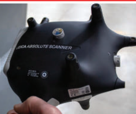
The Leica Absolute Scanner is a handheld device for 3D scanning where high productivity is a priority. Working with the Leica Absolute Tracker AT960 range of high-end laser trackers, it makes possible previously infeasible large-scale 3D digitization. [Exact Metrology]
