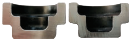
The slim slug process allows for reduction of the slug thickness. In the production of a combination ring 6008 blank, 25 grams of raw material can be saved. [Hatebur]
