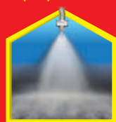
Narrow Angle Flat Fan Spray Pattern
