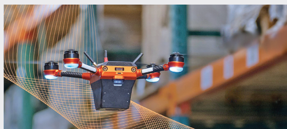
Corvus One warehouse drones autonomously take off and land, charge, and transfer data on premises at the landing pad.
