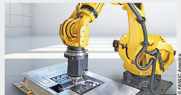
Built for payloads up to 1,100 lb, FANUC's M-950iA/500 serial-link robot offers precise, versatile motion—even in tight spaces.
