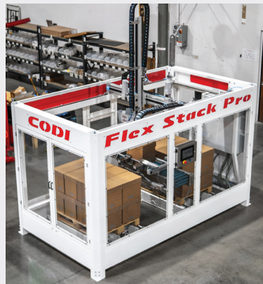
The Flex Stack series of gantry palletizers/ de-palletizers is based on world-class Festo mechatronic technology. © CODI Manufacturing
